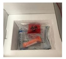
7.2.8 Put a second CRT gel pack on top of the sample.
