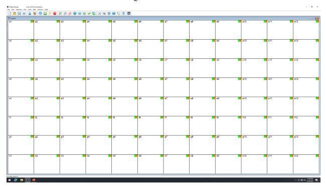
8.3.7 To add information on cell lines used, cells/well, and treatments, click on the Tools menu, click Plate Layout, then click Edit Layout. This will open the Wells Properties window.
