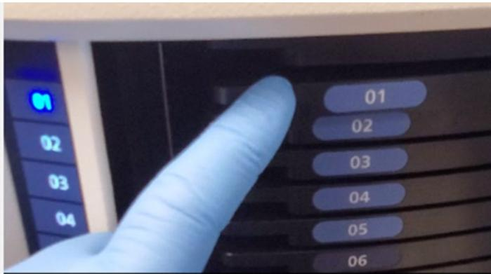
12. Close the Axioscan door by pressing the “open/close” button as shown below.
