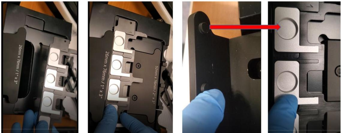
4. Push forward handle on the slide of the tool as shown in (A) below. This will open the individual slide locations as shown in (B) below
