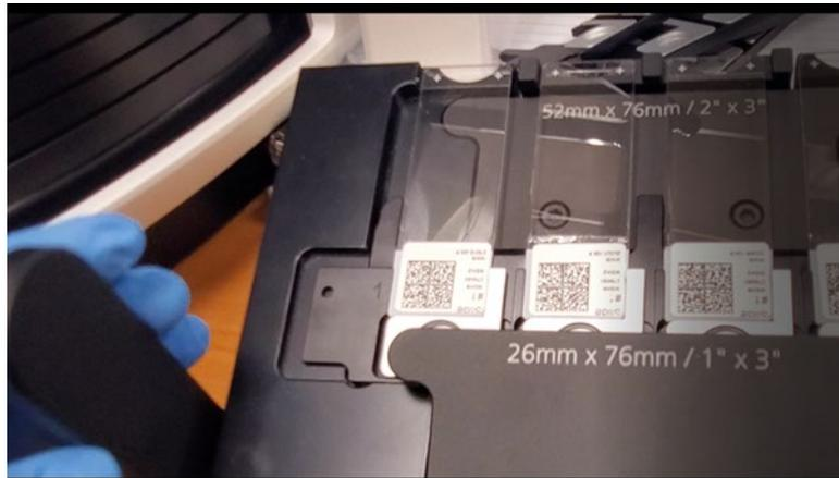
9. Pull the left corner of the tray out to open a slide tray as shown in (A) below. Image of an open tray is shown in (B) below.
