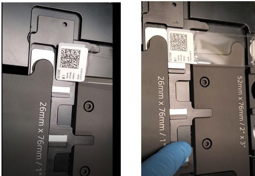
7. Record slides and corresponding locations in the Excel Axioscan Slide Tray Template as slides are being added to the slide holders. An example is shown below.
