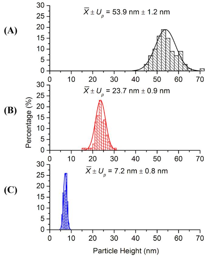
**Figure 4.** Histograms for 60 nm (A), 30 nm (B), and 10 nm (C) nanoparticles (nominal).
