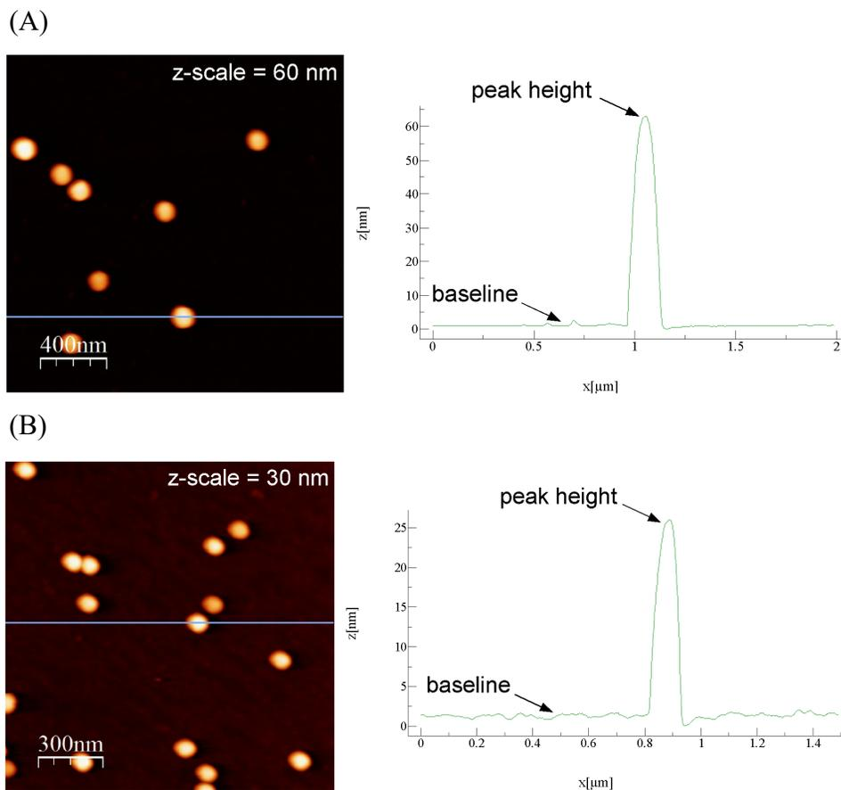
**Figure 3.** AFM images and cross-sections for 60 nm (A) and 30 nm (B) nanoparticles (nominal). The difference between the peak height and the average baseline (from both sides of the nanoparticle) is the particle height.
