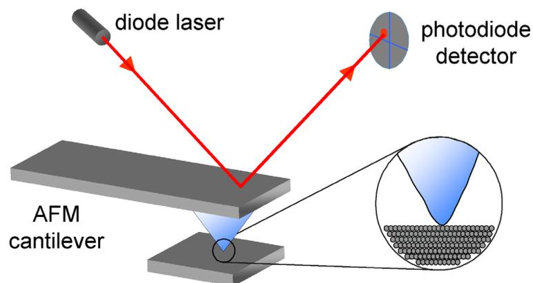
**Figure 1.** Schematic diagram of an AFM. A laser beam is focused on the back of a cantilever that has a tip that interacts with a surface; the beam reflects into a four-quadrant photodetector. Normal forces between the tip and surface deflect the cantilever up or down. Lateral forces twist the cantilever left and right. These deflections are measured by monitoring the deflection of the reflected laser.
