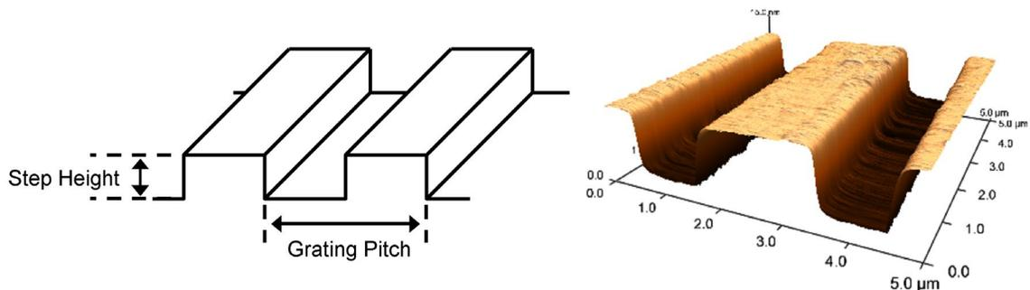
**Figure 2.** Schematic diagram and AFM image of a calibration grating consisting of an array of rectangular SiO<sub>2</sub> steps on a Si wafer. For this particular grating, the step height was certified to be 19.5 nm ± 0.8 nm.
