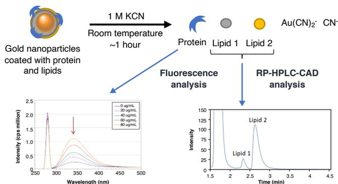
Colloidal gold nanoparticles are dissolved using KCN to afford free protein and lipid surface ligands. The resulting solution is analyzed for concentration of individual components.
