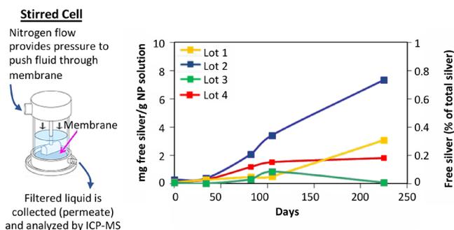
Stability assessment of four batches of colloidal silver nanoparticles as determined by free silver concentrations. Stirred cell filtration was used to separate free silver from nanoparticle silver. The permeate silver concentration was measured by ICP-MS.
