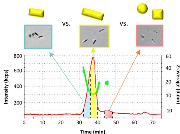
Purity assessment of PEGylated gold nanorods as defined by the presence of non-rod shaped particles. Particles were separated by AF4-DLS, and collected fractions were analyzed by TEM to confirm shape. Adapted from Anal Bioanal Chem, 2020, 412(2), 425-428.
