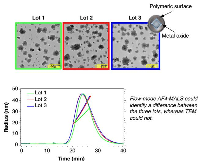
Representative TEM images (top) versus flow-mode AF4-MALS (bottom) measurements for three batches of a polymer coated metal oxide formulation. In this case, AF4-MALS was better suited in assessing the size distribution and differences between these three lots. Adapted from J Control Release, 2019, 299, 31-43.
