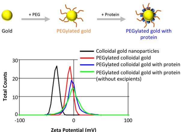
Monitoring the reaction progress of PEG and protein grafting to the surface of colloidal gold nanoparticles by zeta potential. Measurement conditions were identical for all samples.
