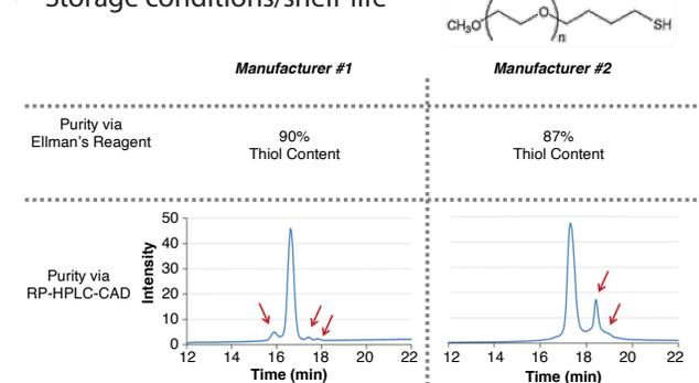
Purity and functionality characterization of 20 kDa mPEG-SH from two manufacturers. Purity was assessed by RP-HPLC-CAD and thiol content by the Ellman's reagent. Adapted from AAPS J, 2017, 19(1), 92-102.
