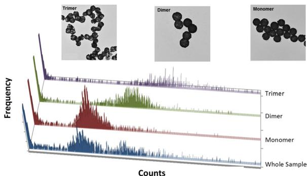
Single particle ICP-MS and representative TEM images of PEGylated core-shell nanoparticles. spICP-MS can resolve the different species in a single run and determine the size of each population.
