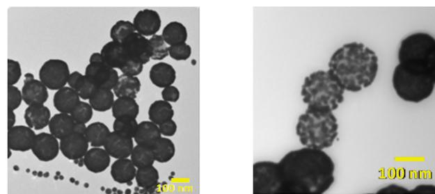
Representative TEM images of gold-core silica-shell nanoparticles. In addition to determining the size distribution, TEM can be used to evaluate morphology and purity assessment. Here, smaller gold nanoparticles and incomplete gold coating were observed. Elemental composition was confirmed by energy dispersive spectroscopy (EDS).
