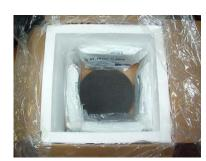
Figure 4: Place one -20 °C frozen 4-lb freezer brick in plastic bucket.
